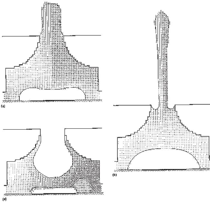
**Figure 2** Simulation plots of ink droplet ejection (reprinted by permission from *HPI*, May 1985: 26). The upper left illustrates 5  $\mu$ s after bubble formation and the right illustrates 15  $\mu$ s after formation. The ink droplet is about to separate in the right illustration. The lower left illustrates the bubble collapse that was to cause the cavitation difficulties.
