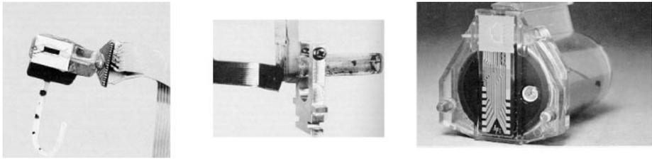
**Figure 3** From left to right, the first seven-orifice Corvallis prototype; the first prototype placed within an existing HP printer; and the HP Model 2225 Printer thermal ink-jet printhead (reprinted with permission from *HPJ*, May 1985: 5, 6 and 10).
