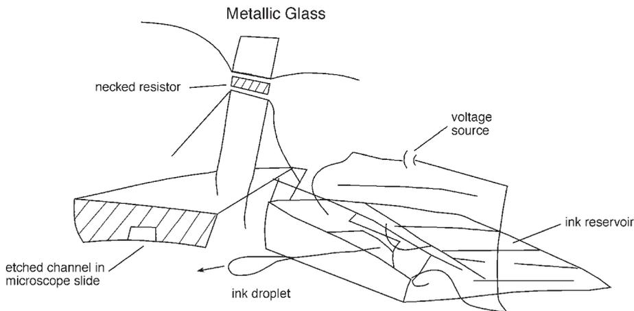
**Figure 1** John Meyer's drawing of the metallic glass prototypes (J. Meyer, personal interview). John Vaught would first deposit metallic glass on the microscope slide and then etch it down to a necked resistor. He would then etch out a channel in another slide and fill it with ink. Finally, he would place the first slide above and perpendicular to the direction of the ink droplet. Ink drops would eject when he subjected the necked resistor to a voltage pulse.
